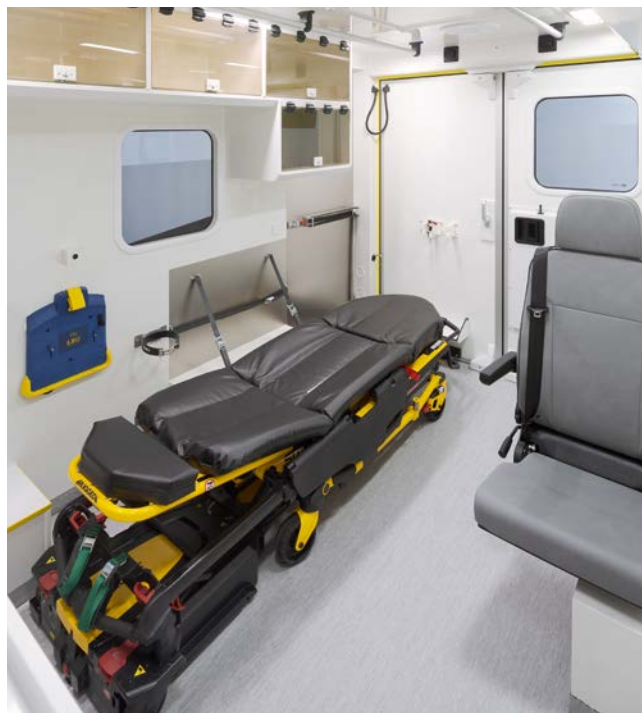
The saloon interior is manufactured from a lightweight rigid PVC with high visibility edging, highly resistant to bacteria and disinfectant and free from organic material.
