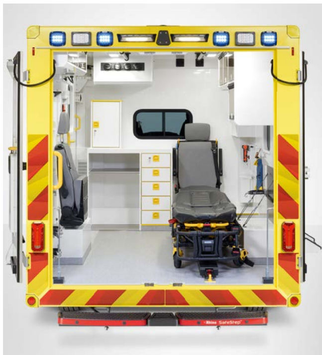
The auto loading stretcher system reduces muscular skeletal injuries, servicing costs and VOR.
