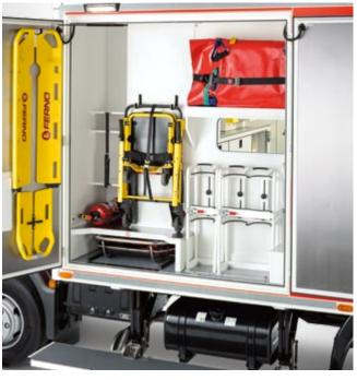
Outside storage compartments and access flaps offer a lot of additional space. Foldable side step for an easy access to the special equipment.
