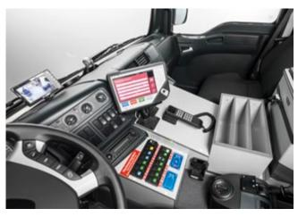
The centre console in the driver's compartment incorporates communication technology, control unit for the warning device and a freezer compartment.
