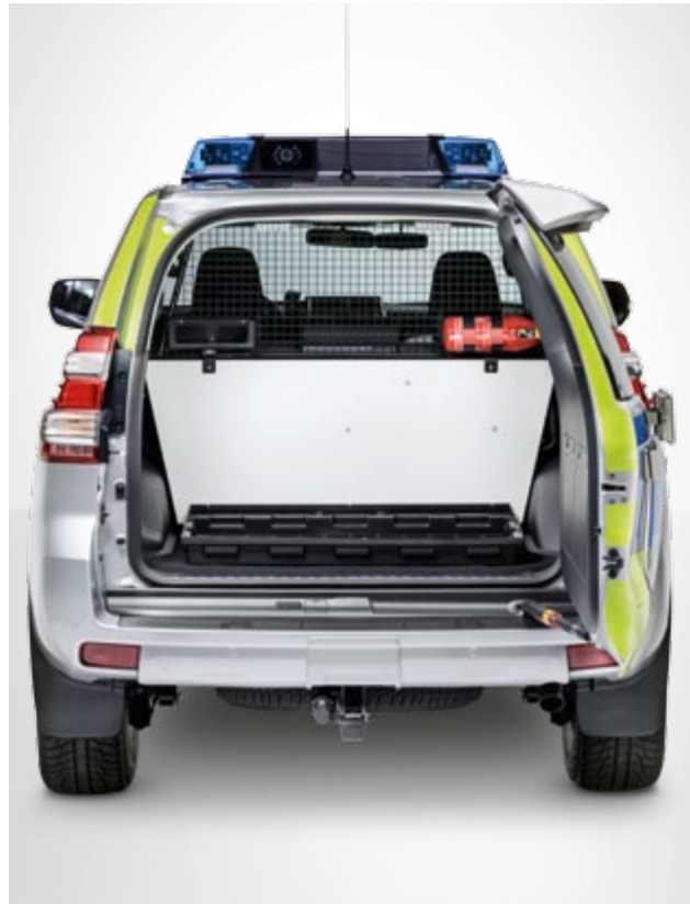
The ceiling-high separation grid and the anti-slip coated container ensure a secure fixation of the material in the rear end of the vehicle.
