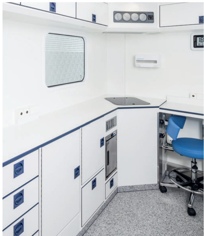
The wash basin can be easily covered to make additional work surface.
