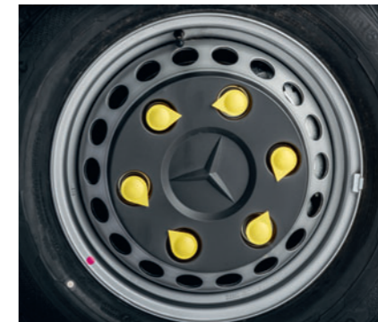
The wheel nut marking shows whether the wheel nuts have been tampered with.
