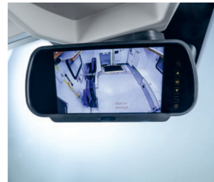
In place of the rear-view mirror, the driver sees the camera view in the patient's room.
