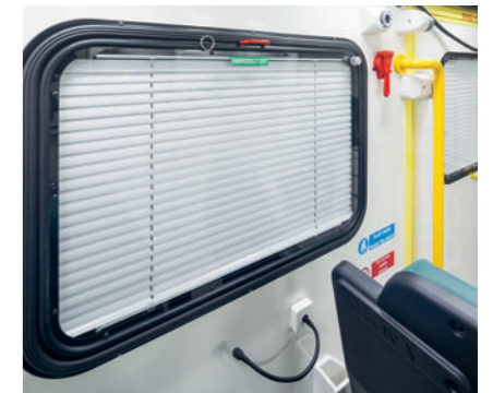
The safety windows resist penetration from the outside. In case of danger, however, they can be easily opened from the inside.
