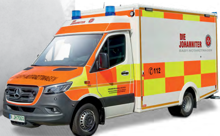
The base vehicle is a Mercedes-Benz Sprinter of the VS30 model generation.
