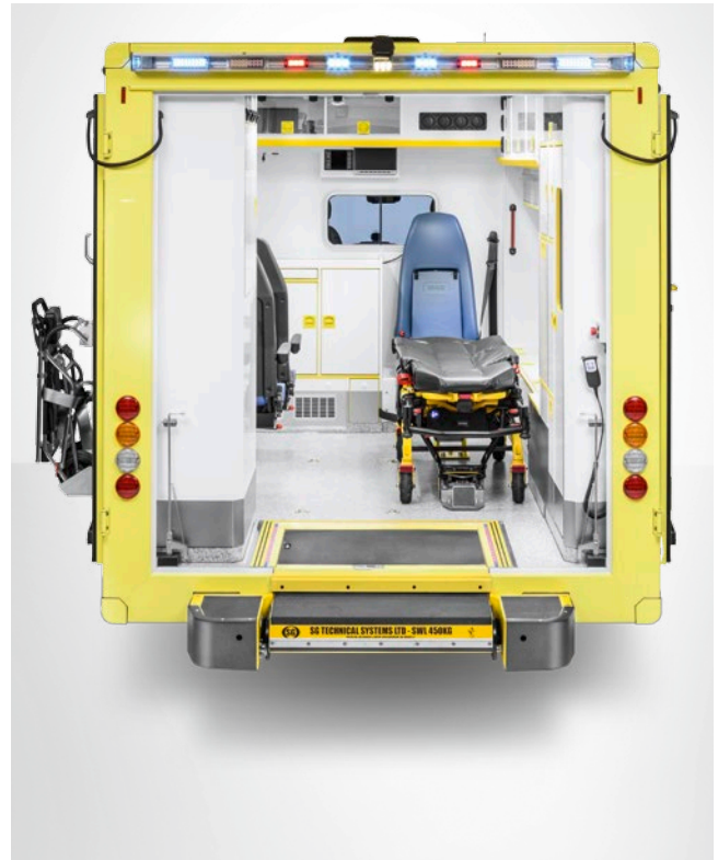
With a greater internal width of 100mm compared to the Fiat panel van, it is possible to enter the vehicle with a carry chair without having to stow away the n/s seats.
