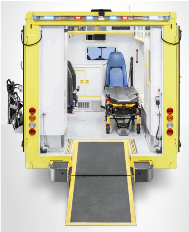
Easy load powered 450kg SWL wedge ramp. To aid loading the vehicle is also fitted with an electrically operated winch.
