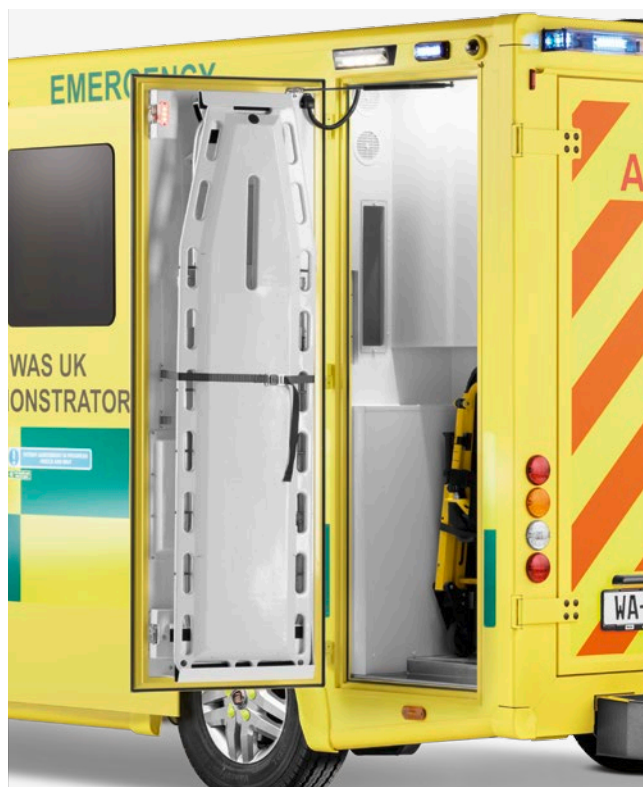
An external locker designed for quick and easy access to medical equipment.
