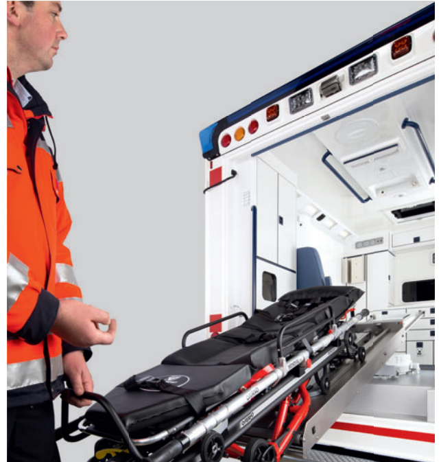
The WAS Multi-Load Assist is activated after connecting the stretcher to the move-in system.
