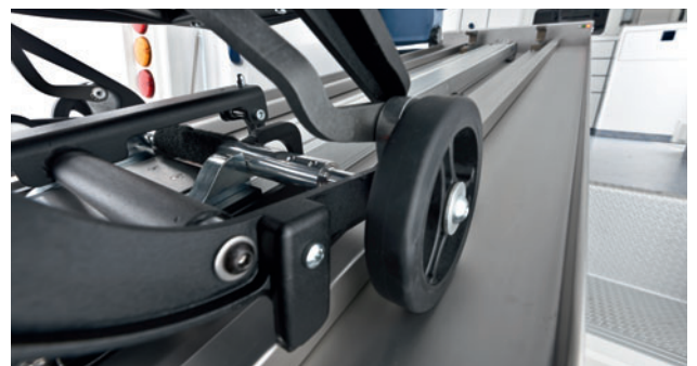
The move-in carriage which is suitable for any stretcher system assures a safe locking.
