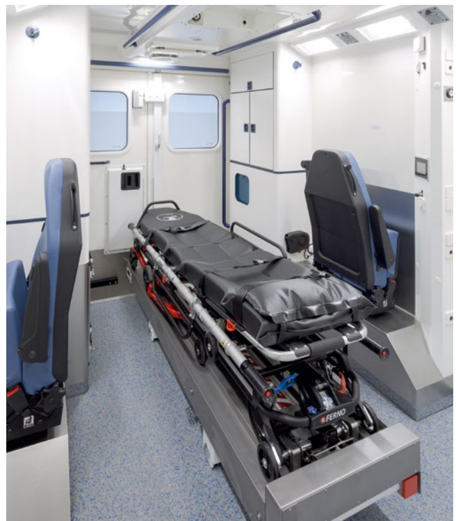
The seats can be folded and rotated for optimal interior arrangement during patient treatment. The ambulance table with stretcher can be moved from its central position to the right and left.
