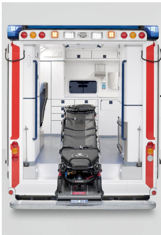
Optimal use of space ensures the greatest possible freedom of movement. The rear frame allows the doors an opening angle of 270° and the integrated step box ensures safe exit and entry thanks to the uniform height of the steps.
