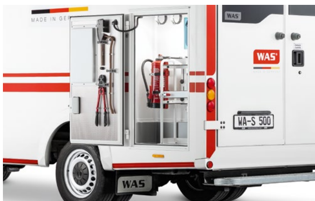
Compact and ergonomic: Oxygen supply and rescue tools in the large exterior storage compartment.
