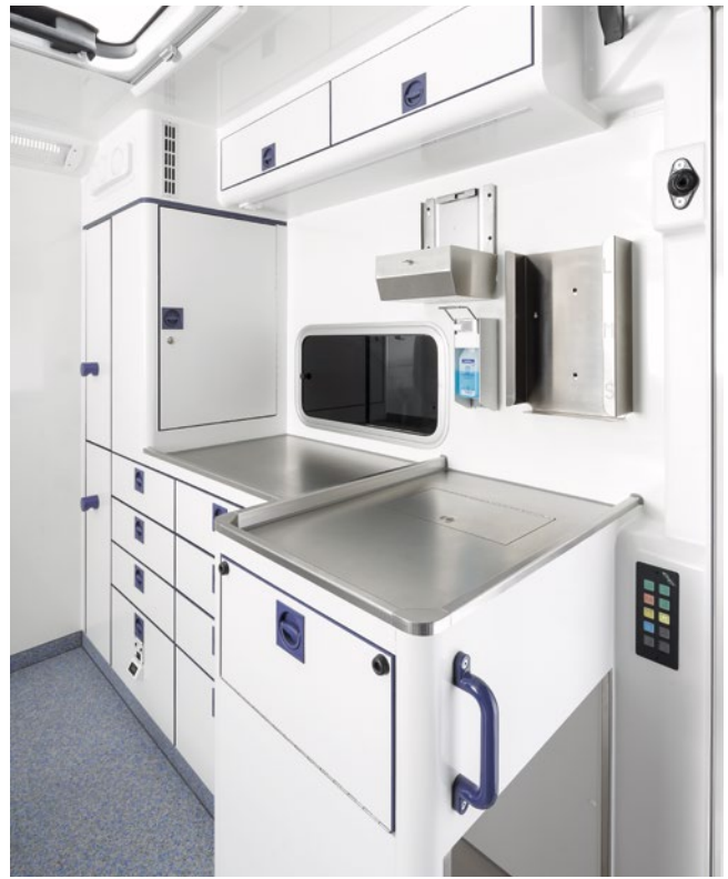
The rounded edges of the furniture provide greater safety to people in the vehicle and allow for easier cleaning and disinfecting.
