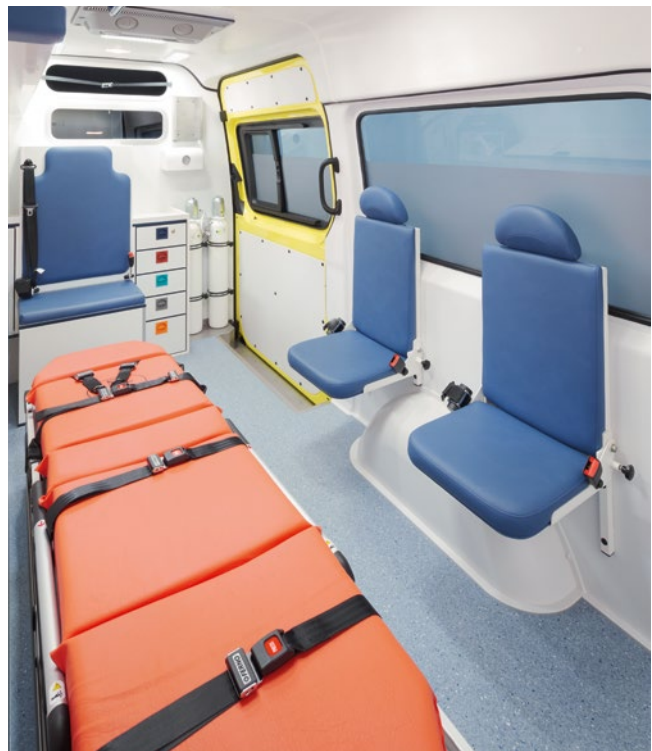
Two foldable seats on the right side for paramedics or family members.
