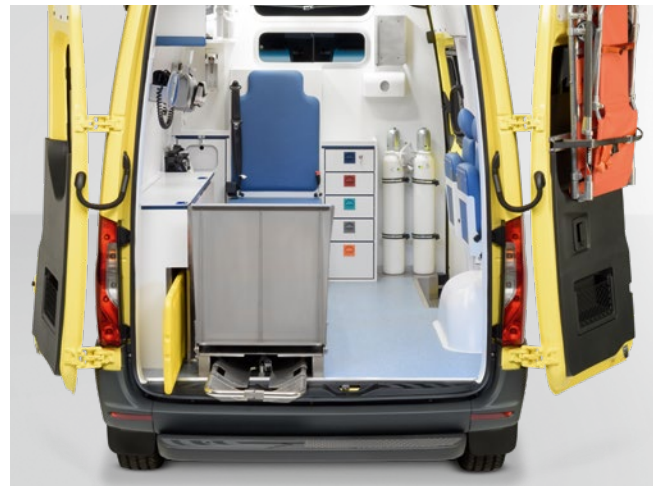
Scoop can be stowed under the stretcher platform, carrying chair is easily accessible at the rear door.
