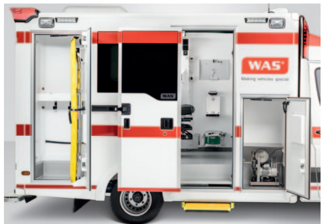
The external access hatches ensure time-saving removal of equipment.
