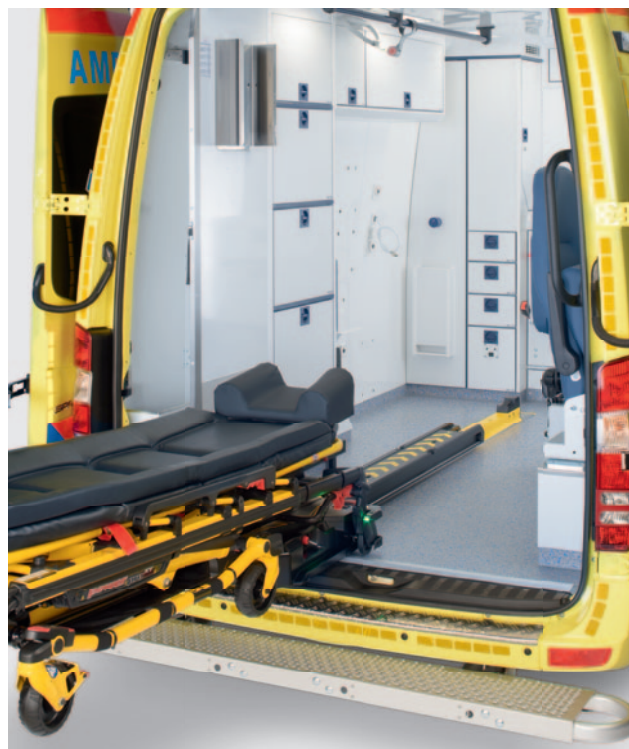
The power-LOAD wheeled stretcher system ensures safety and ergonomics when loading the ambulance.
