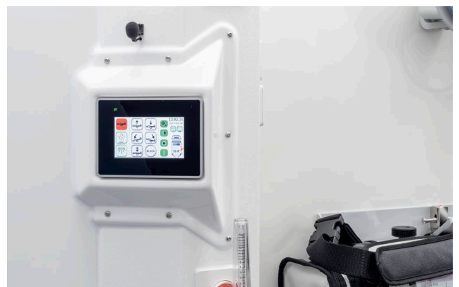
Touchpanel to control all functions of the saloon.
