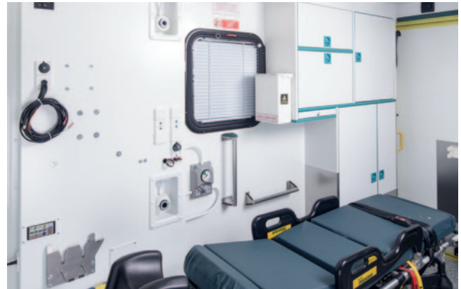
The Mediboard on the side wall allows direct access to medical technology.
