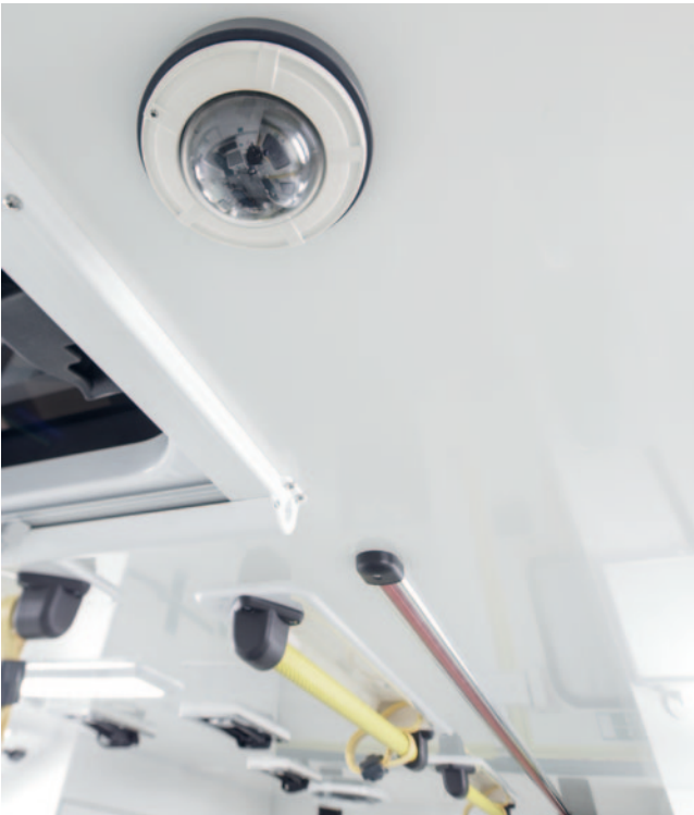
Multi point panic strips to activate internal video surveillance system and to alert the driver.
