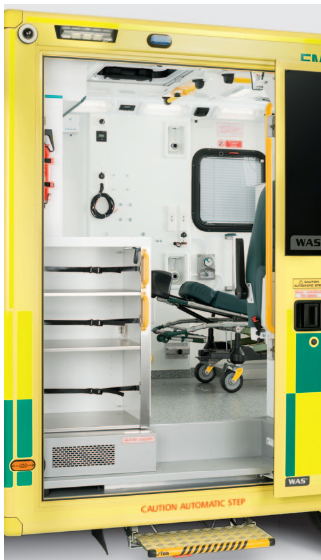
Side sliding door provides maximum access to the patient compartment when space is limited and allows emergency removal of stretcher.
