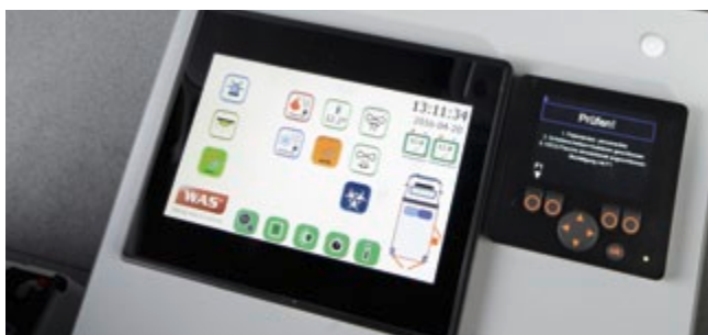
A large control panel with 7" touch screen and the control system for the WAS SanSafe disinfection unit are located in the centre console of the driver's compartment.
