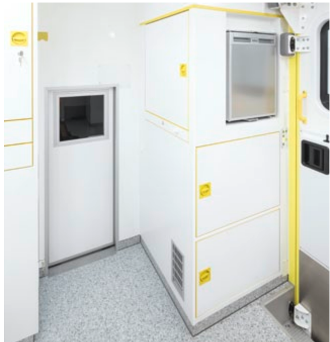
Sliding door between the patient compartment and the driver's compartment for an easy move of the rescue team between these two areas.
