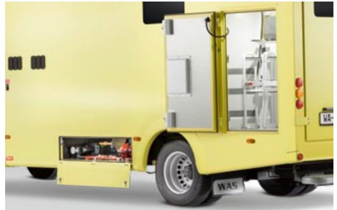
Compact and secure: Oxygen supply in the exterior storage compartment, rescue tools in the under-floor compartment.
