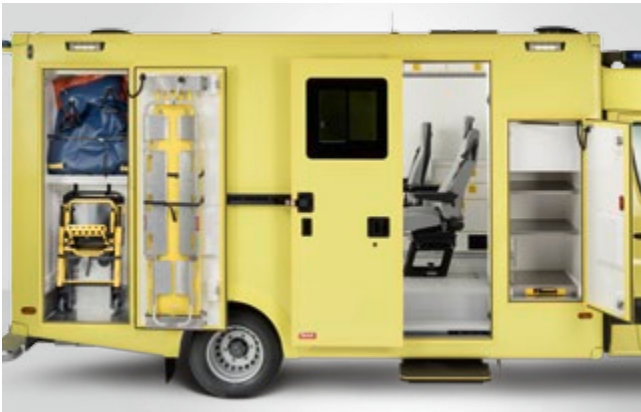
Carrying chair, vacuum mattress, scoop stretcher and spine board are securely fixed but can be easily removed.
