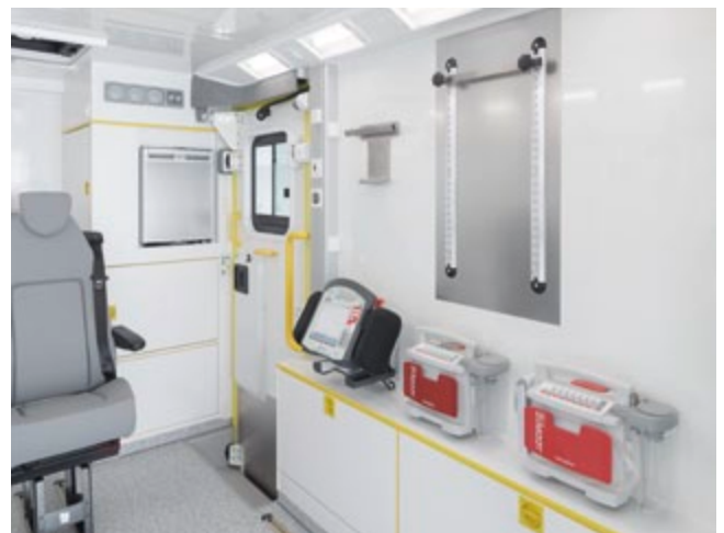
Airline rails in the floor and on the side walls for a secure fixation of external equipment.
