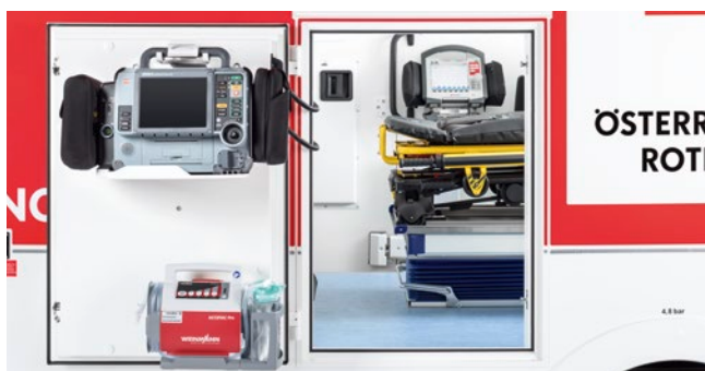
Thanks to the functional outside door, the rescue team can easily access the medical equipment, without entering the patient compartment.
