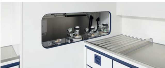
The oxygen and compressed air supply system is suitable even for long transports between hospitals.
