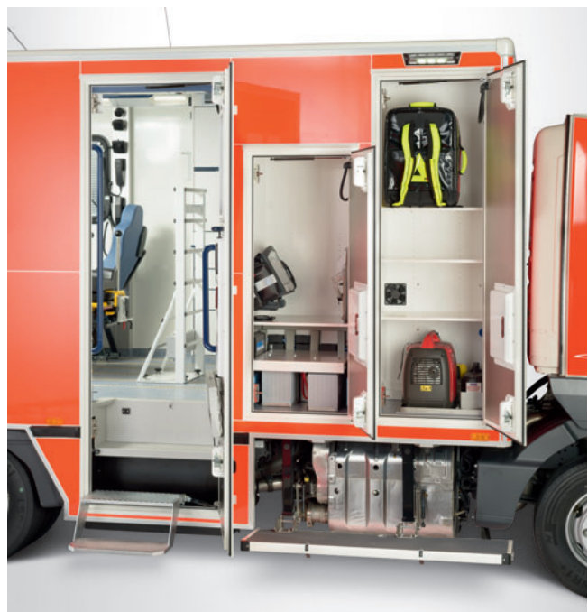
Outside storage compartments and access flaps offer a lot of additional space. Foldable side step for easy access to the special equipment.
