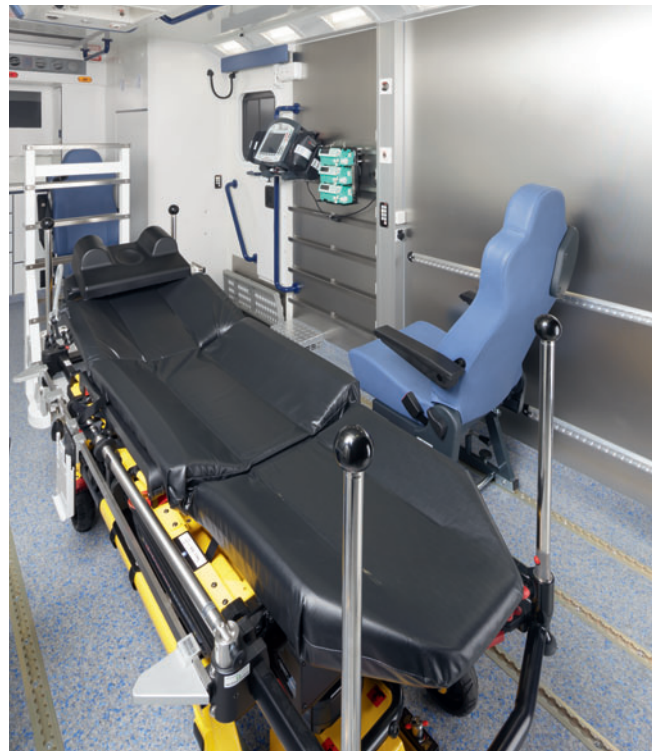
The patient compartment is adapted to various bariatric or intensive transport systems, and offers enough room for even complex medical equipment.
