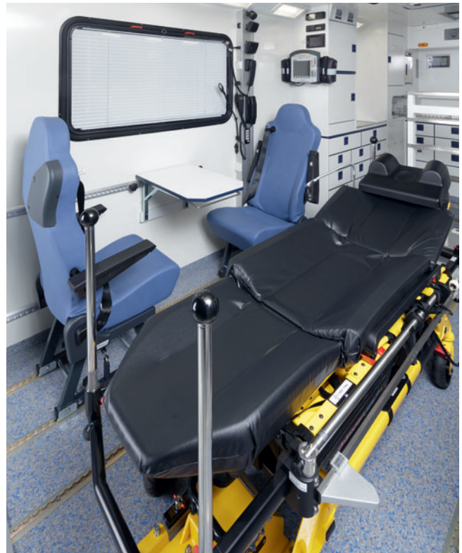
Attendants seats fixed on airline rails and working tables for a maximum of flexibility and comfort.
