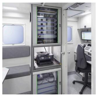
A rack system 19" to accommodate the communication and network technology.
