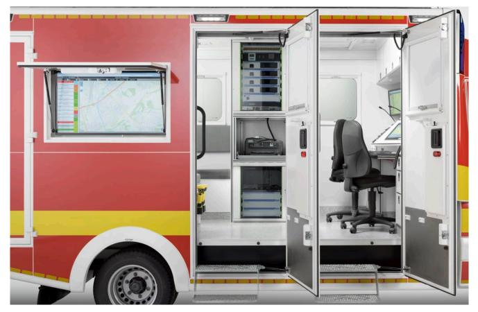
The communication section and the office section are connected with a sliding door. A flat screen 32", fixed behind an access flap, transmits operational information to outward.
