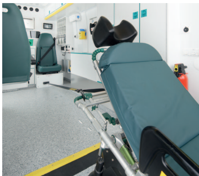
Stretcher winch to loading and unloading of patients both in carry chairs and stretcher.
