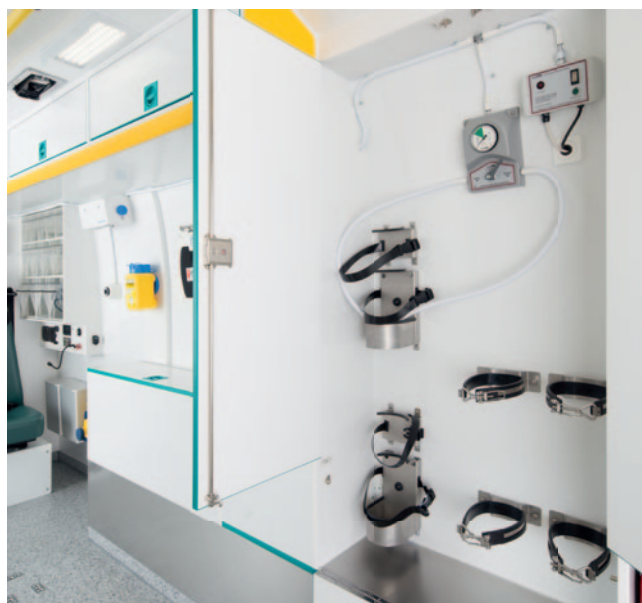
Locker for multiple gas cylinders.
