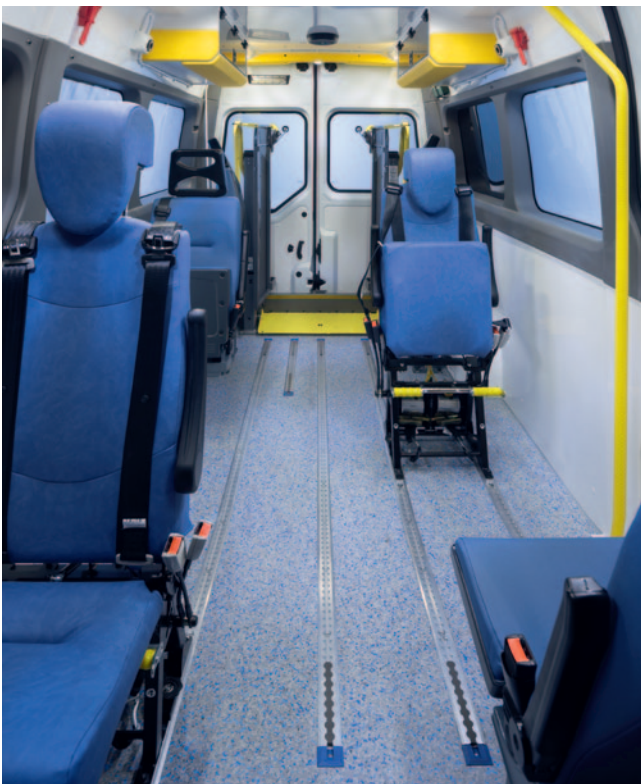
The removable and fixed seating configuration allows transportation of up to 6 walking patients or 4 walking patients and 2 patients in wheelchairs.
