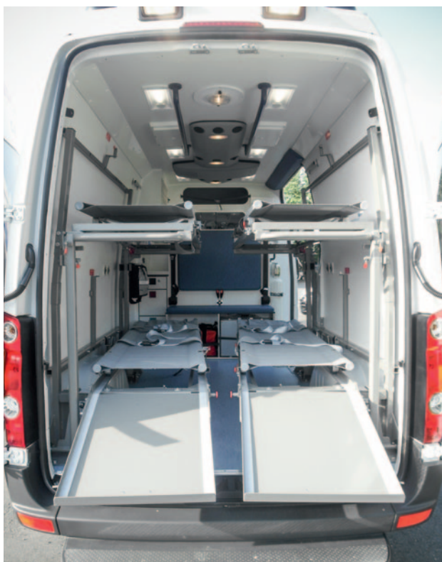
The stretcher brackets can be lowered to enable ergonomic loading.
