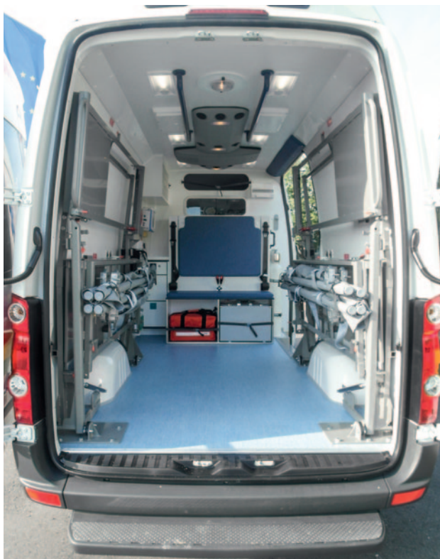
The stretcher brackets to the left and right can be folded up against the sidewalls to maximise space.
