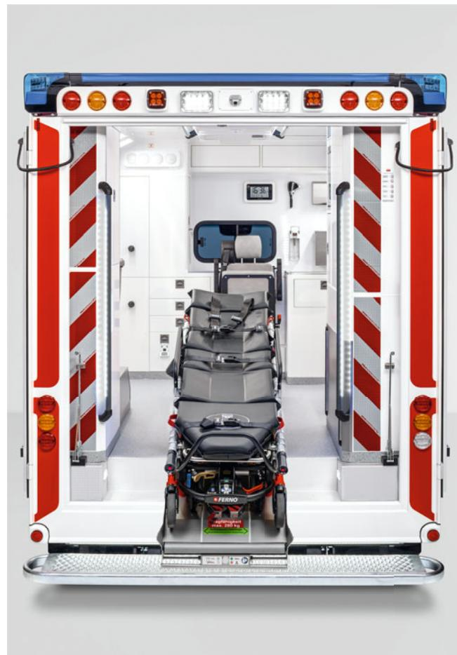
The back-friendly move-in assistance WAS Multi-Load Assist has been developed for all common roll-in stretcher systems.
