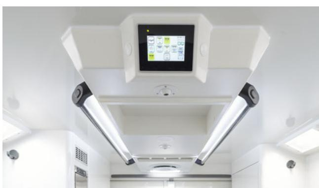
The ceiling centre is used to contain medical equipment, energy and oxygen supply as well as the touch screen used to control the ambulance table and the heating/air conditioning system.
