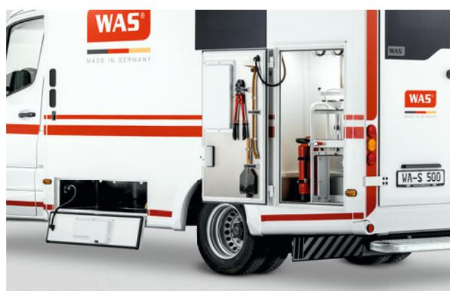
Compact and ergonomical: Oxygen supply and rescue tools in the large exterior storage compartment. The underfloor compartment offers additional storage space.
