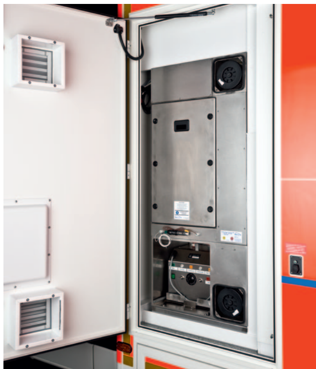
Air cleaning system with integrated fumigation (filtration system according to HEPA H14).
