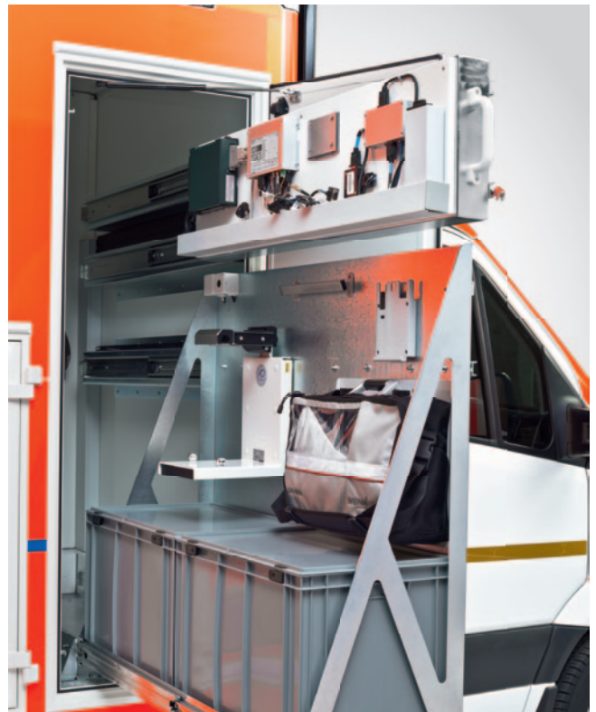
Easy access to medical equipment and protection clothing via heavy duty drawers.
